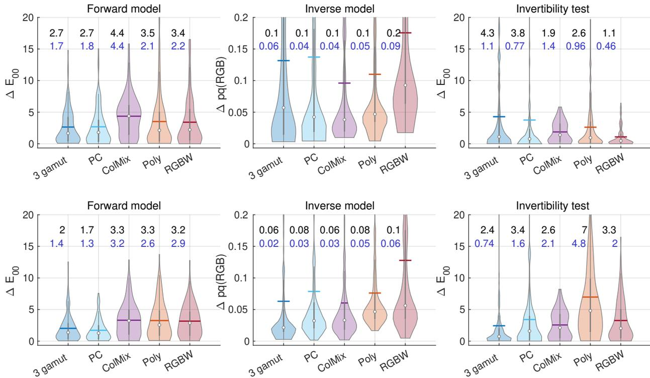
**Figure 2.** The distribution of errors for the G1 (top) and G2 display (bottom). The models are: 3-gamut, PLCC-based compensation (PC), Colour mixing (ColMix), Polynomial regression (Poly) and RGBW gamut. The white circle in each violin plots are the medians and the horizontal dash are the means. The black text at the top left of each violin is the mean, the blue text are the medians.
