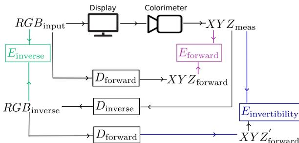
**Figure 1.** Model validation flowchart.  $D_{forward}$  represents the forward models and  $D_{inverse}$  represents the inverse models.  $E_{forward}$  is the forward model error,  $E_{inverse}$  the reverse model error, and  $E_{invertibility}$  is the invertibility test error
